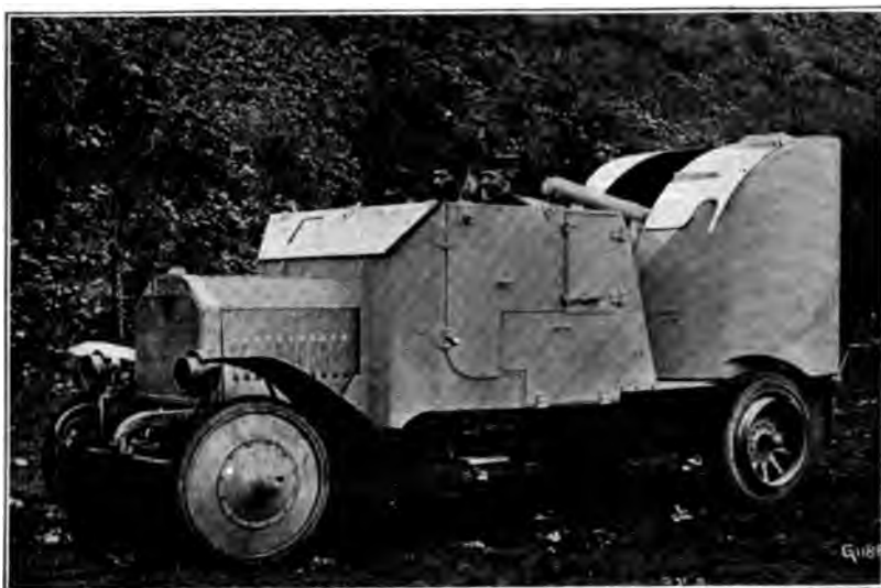
Fig. 47. Krupp Guns for Protection Against Air Crafts
